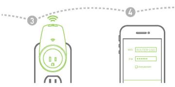
Plug NEO Switch into a power outlet, then press ON/OFF button for 5 seconds and release it. The Wi-Fi indicator light will flash quickly. NEO Switch is now ready for synchronization.
